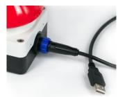
This device is intended to be used with USB hosts or USB hubs. Connecting the device to equipment that does not adhere to the USB standard may damage the device.
