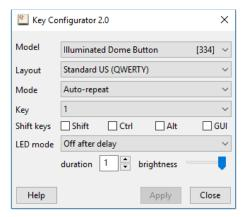
The utility configures only a single button at a time. The serial number, at the right of the model name, shows which button is being configured. The last three digits of the serial number are also printed on the bottom of the USB button itself.
